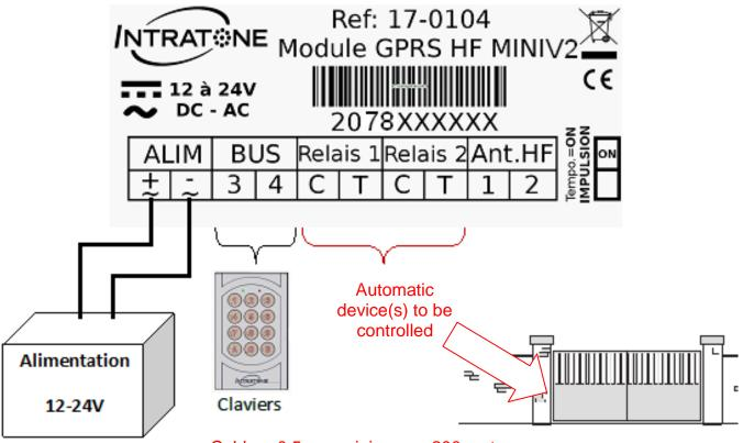
Cable Ø 0.5 mm minimum – 200 metres Relays (1a max): specifically for garage or car-park doors. To power electric or magnet locks, an additional 5a relay must be fitted
